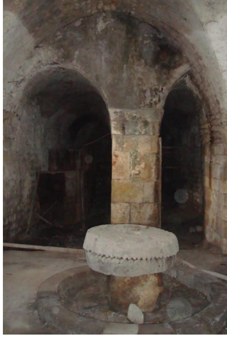
Figure 2.11. Circular crushing stone and its cut stone pool on the floor in Aselci Soap Factory, Antakya
