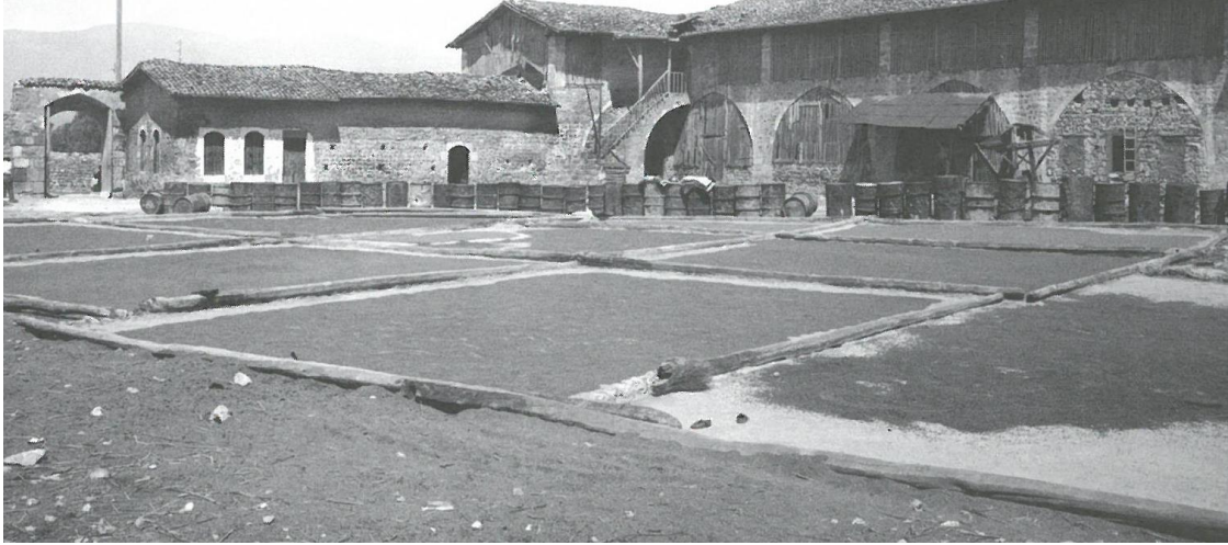
Figure 5.34. The soap molds arranged on the floor of the courtyard of Selahattin Ökten Soap Factory, Antakya
