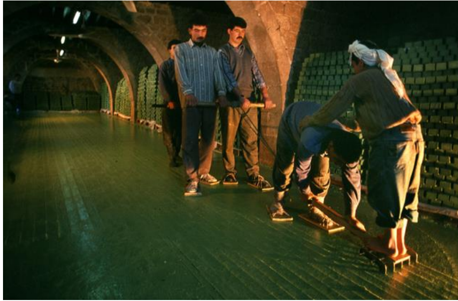
Figure 2.20. Slicing of partially hardened soap in Zenabili Soap Factory in Aleppo, Syria (Source: Touma, 2011)
