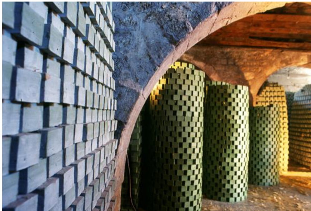
Figure 2.25. Hollow structures of soap bars called as tenanir in Zenabili Soap Factory in Aleppo, Syria (Source: Touma, 2011)
