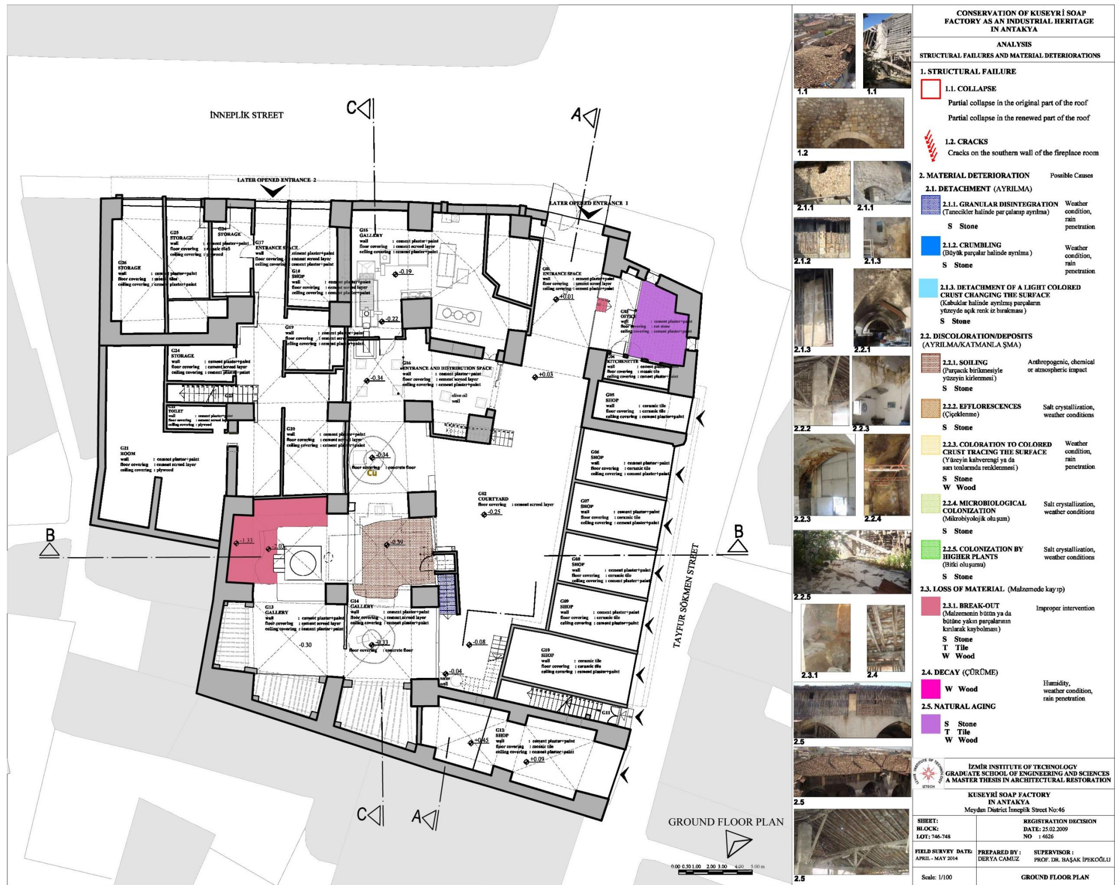
Figure C.5.2. Structural failures and material deteriorations – Ground Floor Plan
