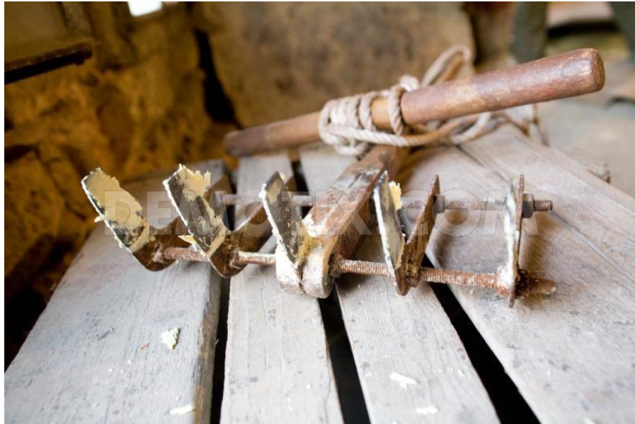
Figure 2.19. A wooden stick with sharp metal pieces attached at the bottom for cutting of partially hardened soap (Source: Sons of Sadik Adra, 2010)
