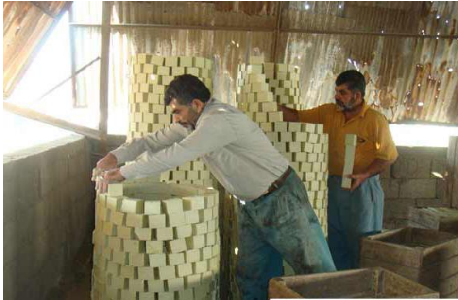
Figure 2.24. Hollow structures of soap bars called as tenanir in Sadein Soap Factory in Tripoli, Lebanon (Source: Sons of Sadik Adra, 2010)
