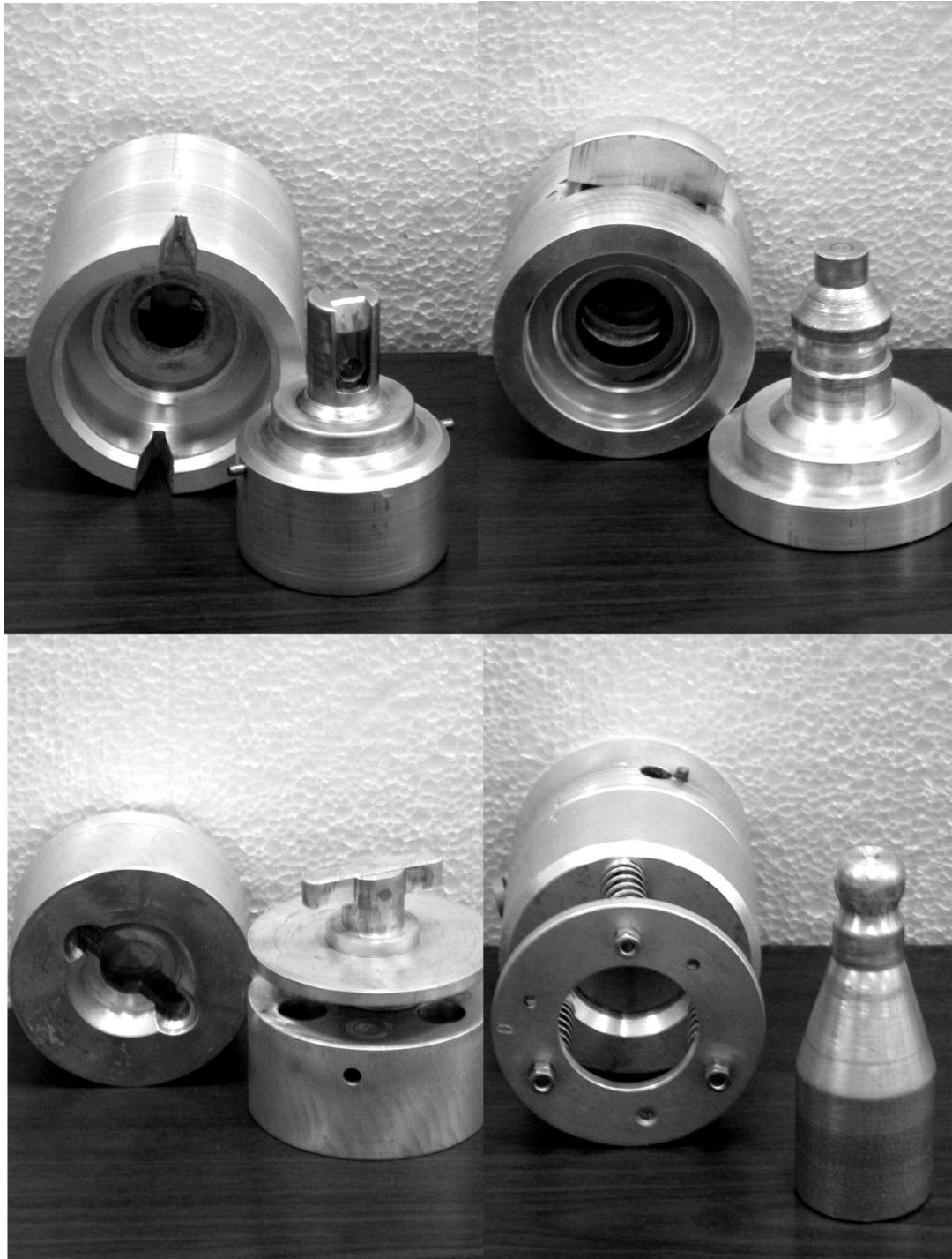
Fig. 22. Male and female parts of the four manufactured joints.
