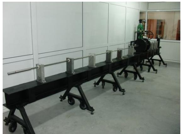
**Figure 3.** Split-Hopkinson Pressure Bar apparatus
