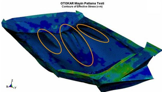
**Figure 12.** Stress concentration on the V-hull
