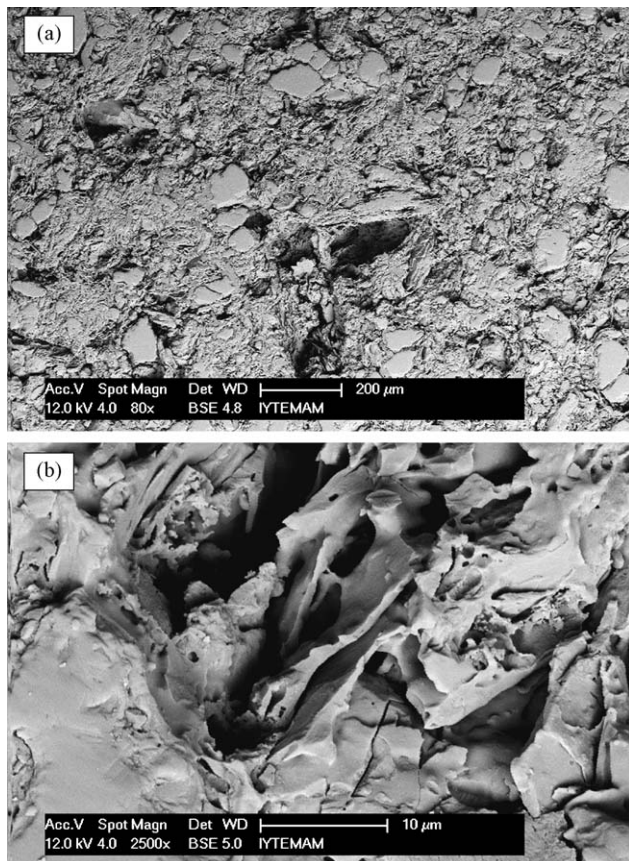
Fig. 8. The SEM images of fired bricks without residue, at various magnifications.
