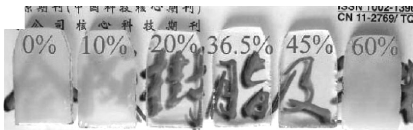
Figure 20. Micrographs indicating the transmissive properties of epoxy-resins blended with TiO 2 @SiO 2 (core/shell) nanoparticles at different thicknesses of the TiO 2 shell. When index matching between particles and matrix is reached, optimal transmission is observed. Data reprinted from ref. [112] with permission of ACS.
