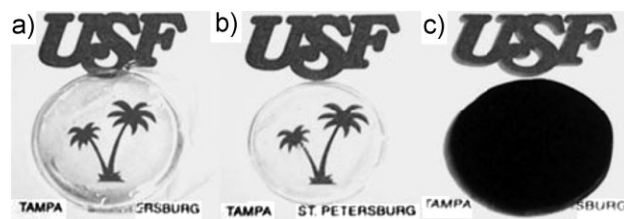
Figure 5. Photographs of discs of different PMMA/SWNT nanocomposites: (a) obtained by in situ UV light induced bulk polymerization of a colloidal dispersion of SWNTs in MMA, (b) neat PMMA for comparison, (c) PMMA/SWNT composite obtained by melt blending. Reprinted from ref. [69] with the permission of Wiley.
