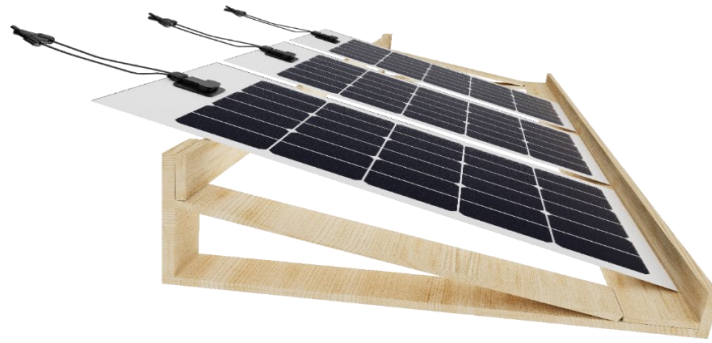
Figure 30 Experimental Setup with 20-Degree Tilt Angle for Photovoltaic Modules.
