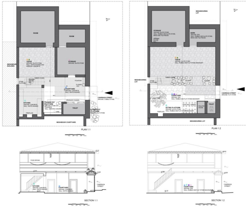
Figure 3. Measured drawings in the current and authentic states in case 1 (Source: Prepared by Author 2024)
