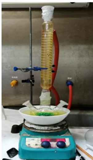
Figure 4.33. Experiment set-up for synthesis nickel hydroxide.
