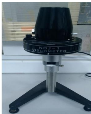
Figure 4.15. The used viscosimeter for optimization of the printable inks.
