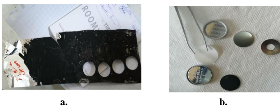
Figure 4.59. a. The applied and cut NMC cathode b. Coincell pieces.
