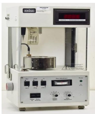
Figure 4.16 The used tensiometer for optimization of the printable inks.
