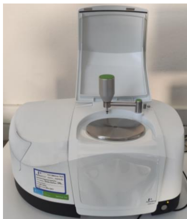
Figure 2.2. ATR-FTIR spectrometer used in the study
