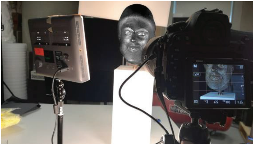
Figure 2. 22. An example of the scanning procedure phase for generating 3D models of ancient works from the Acropolis Museum website (Source: © Acropolis Museum 2024)
