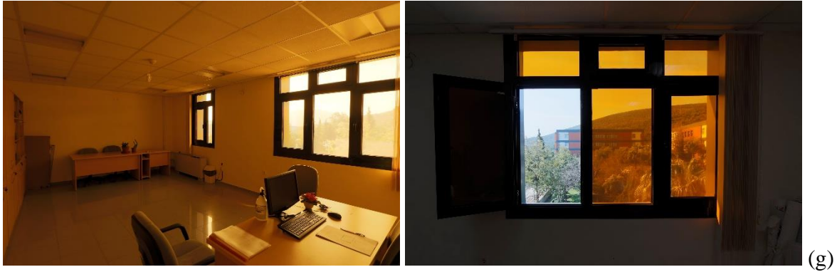
Figure 4.9. Interior view of rooms with different glass types: (a) smart glass, (b) reflective glass, (c) blue solar low-e glass, (d) bronze solar low-e glass, (e) smoked solar low-e glass, (f) orange PV glass and (g) blue PV glass
