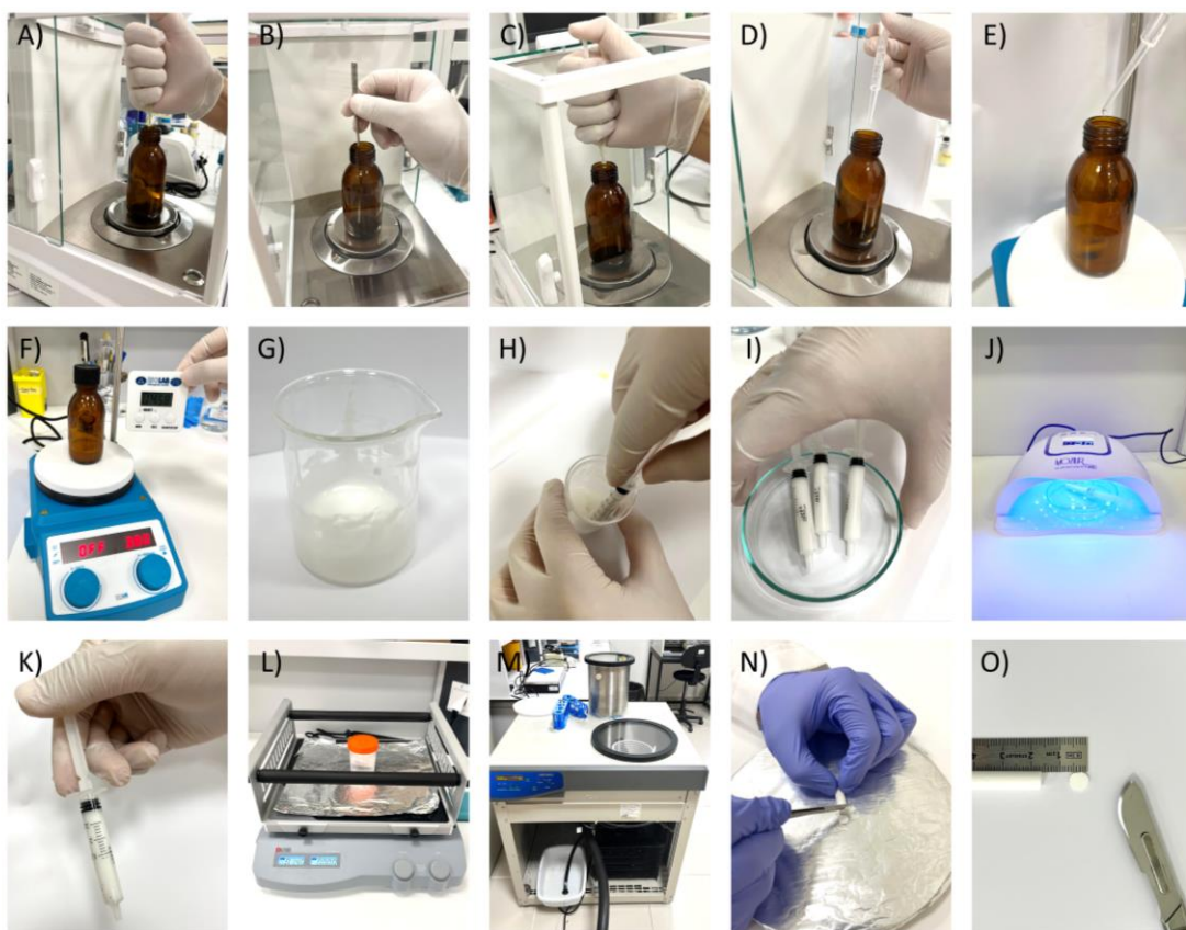
Figure 14. Synthesis process of 4PCLMA-based PolyHIPE via emulsion templating.
