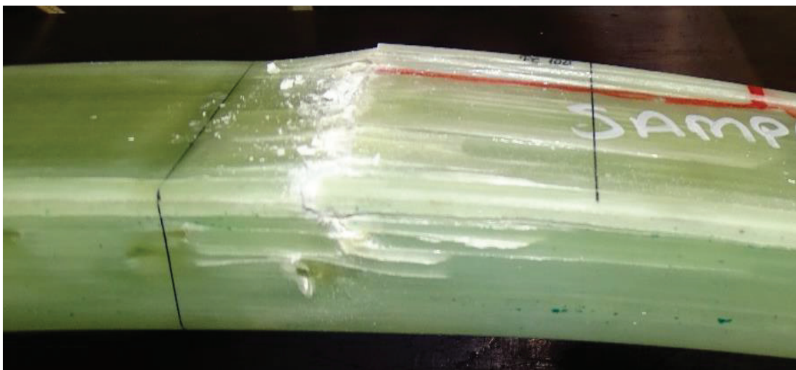
Figure 3.79. Sample#1 Typical Failure.
