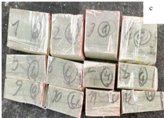
Figure 3.67. Sample#4 FVF Sections. a-Sections of the sample b-Precured sample c- Position of FVF section on the sample's layup.
