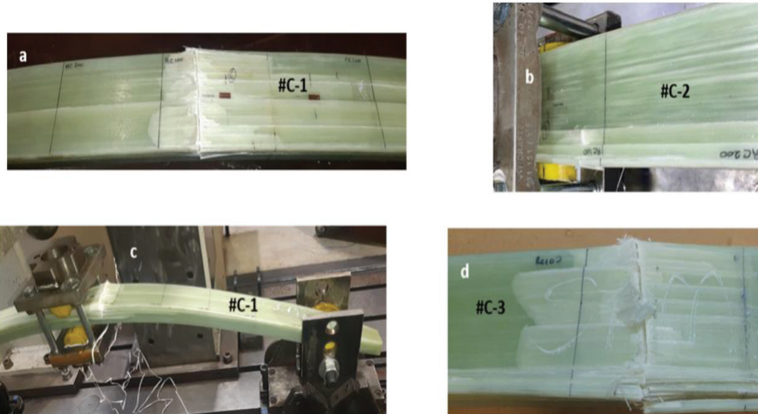
Figure 3.72. Sample #C Fmax Test. a-Sample 1 after the test b-Sample 2 after the test c-Sample 1 after the break at the rig d- sample 3 after the test.
