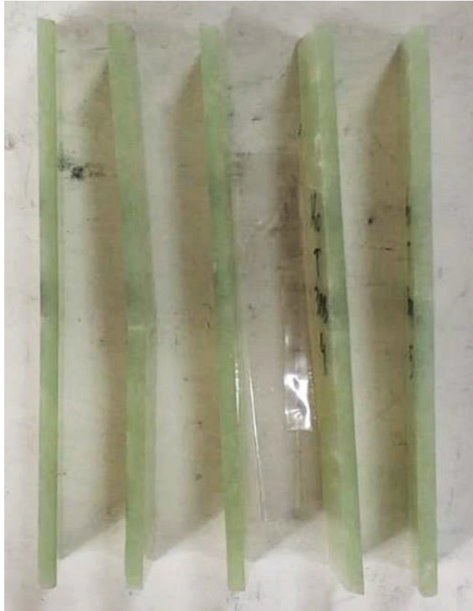
Figure 3.22. Examine the Transverse Three Point Bending Coupons Following the Test.
