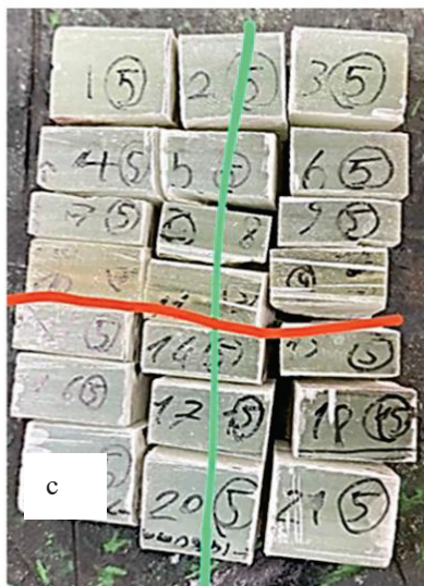
Figure 3.68. Sample#5 FVF Sections. a-Sections of the sample b-Cured sample c-Position of FVF section on the sample's layup
