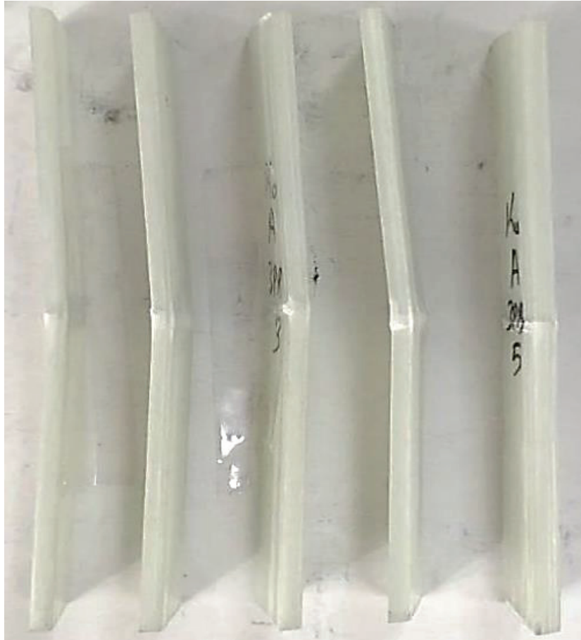
Figure 3.20. Axial Three-Point Bending Coupons After the Test.
