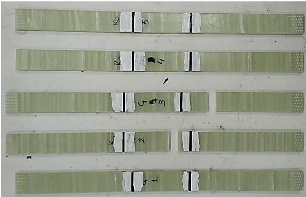
Figure 3.14. Tensile Transverse Test Coupons After the Test.
