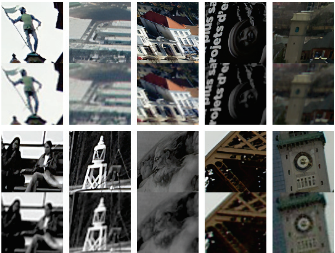
Figure 4.9. Sample Patches from Warped Images: The image patches above demonstrate the results of the proposed warping method, whereas the image patches below show the results of the bicubic warping method.
