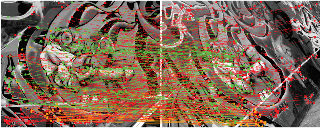
Figure 2.3. Outputs of Feature Matching: SIFT features (centers of the previously detected DoG keypoints and their corresponding descriptor vectors) are matched with their nearest neighbors in descriptor space across images. The search is bidirectional, retaining only mutual matches. Additionally, only the 512 matches with the smallest descriptor distances are kept. Green-marked matches are the best, orange-marked matches are moderate, and red-marked matches are the worst, as compared to the ground truth homography matrix.
