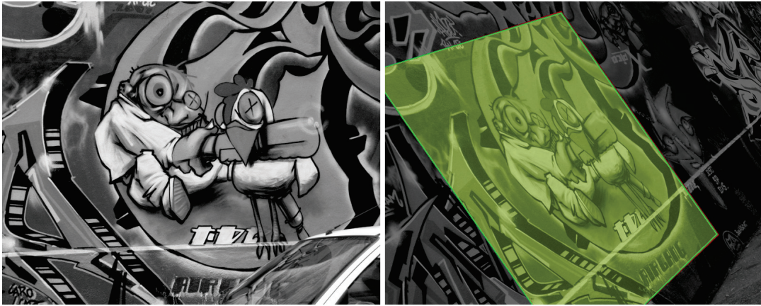
Figure 2.5. Estimated and True Homographies: The corners of the left image were projected onto the right image using both the estimated homography (marked in red) and the true homography (marked in green). The estimated quadrilateral is nearly invisible because it almost perfectly aligns with the true one. Note that neither the automobile visible in the first image nor the ground visible in the second image prevents accurate determination of the camera movement. Since the scene is mostly planar, these elements are treated as occlusions that must be discarded, and local features are capable of handling them effectively.
