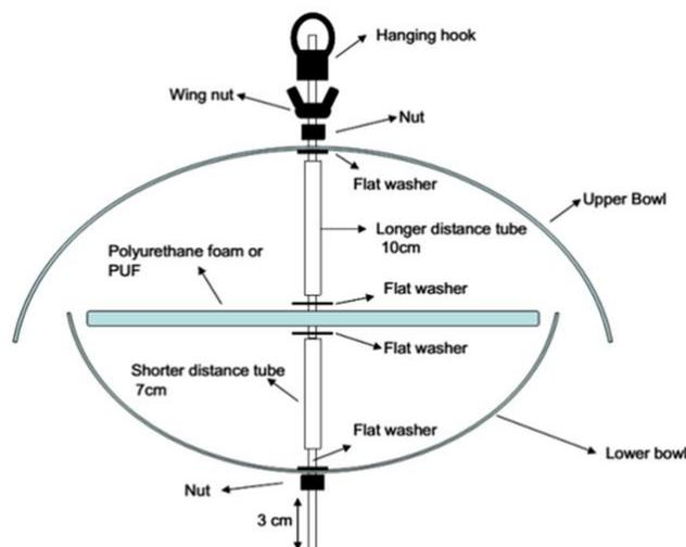
Figure 2.5. Detailed PUF disc as a passive sampler (United Nations Environment Programme, 2017)
