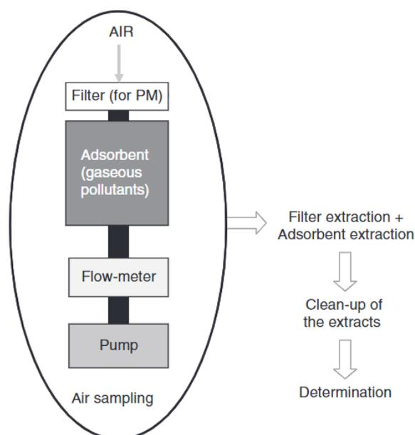
Figure 2.4. The active air sampling device and the analytical steps (Garcia-Jares et al., 2012)
