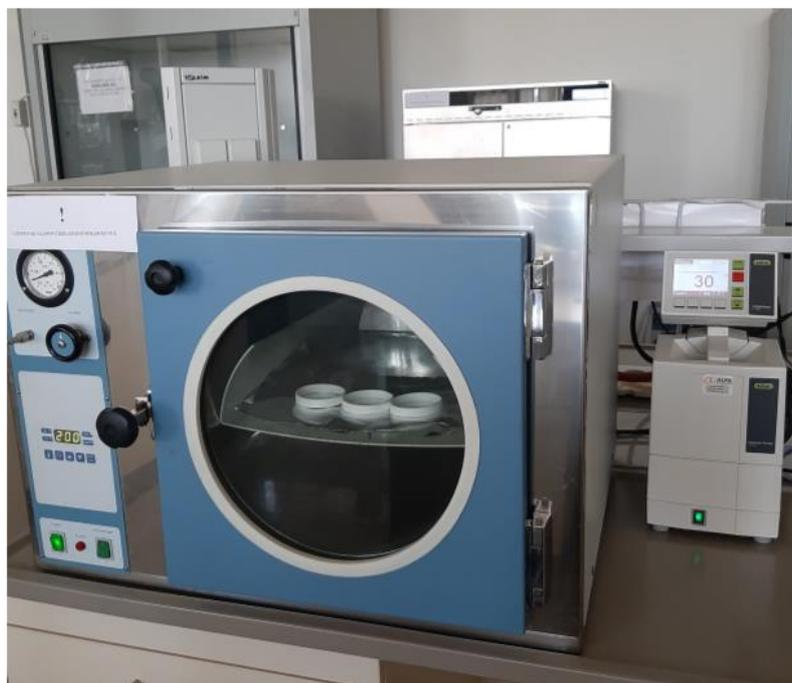
Figure 3.4. Pre-cleaning with vacuum oven
