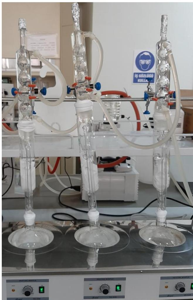
Figure 3.5. Pre-cleaning with Soxhlet system
