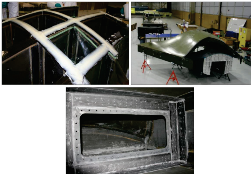
Figure 2.16. Examples of paste adhesive applications; skin paste bonding and paste bonded fuel floor. 81
