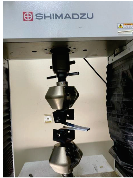
Figure 3.12. DCB test specimen during test.
