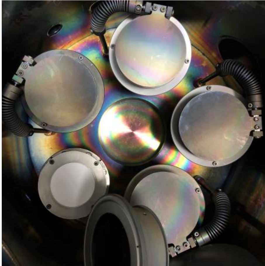
Figure 3.4. Top view of the main vacuum chamber. Scaffolds on the chamber walls and other components were properly cleaned to sustain an ultra-high vacuum environment.
