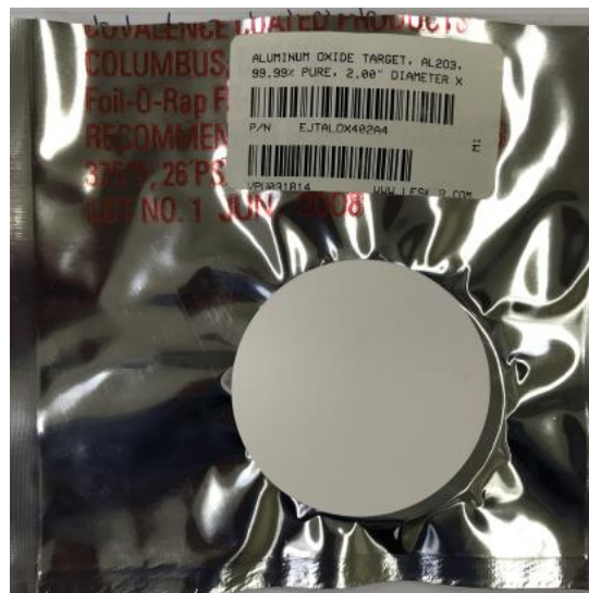
Figure 3.1. New vacuum sealed Al 2 O 3 target. The target is packed under argon gas atmosphere to eliminate and contamination during transport.
