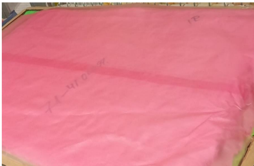
Figure 6. Peel Ply Layup on the fabrics
