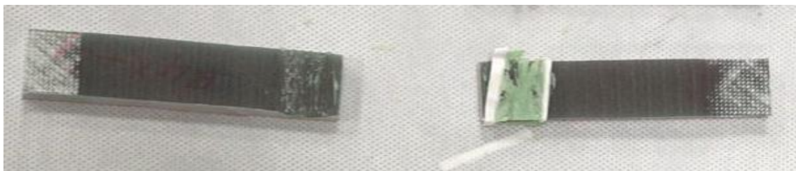
Figure 35. After test images of single lap joints test specimens
