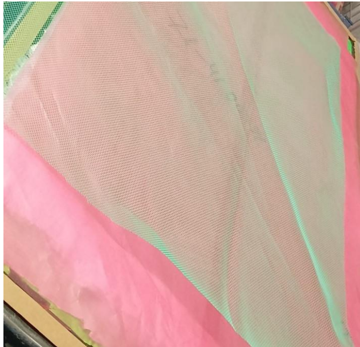
Figure 7. Green mesh is placed on the peel ply
