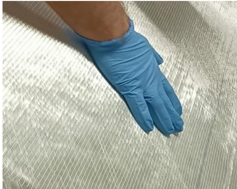
Figure 5. BIAx1000 Fabrics Layup on the mold
