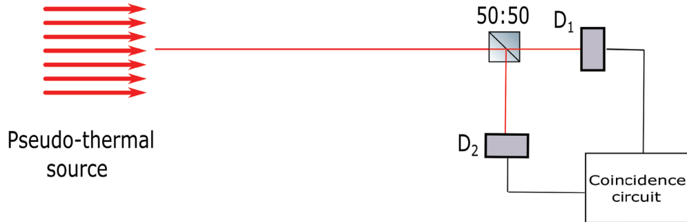
Figure 4.13. Hanbury-Brown-Twiss (HBT) configuration
