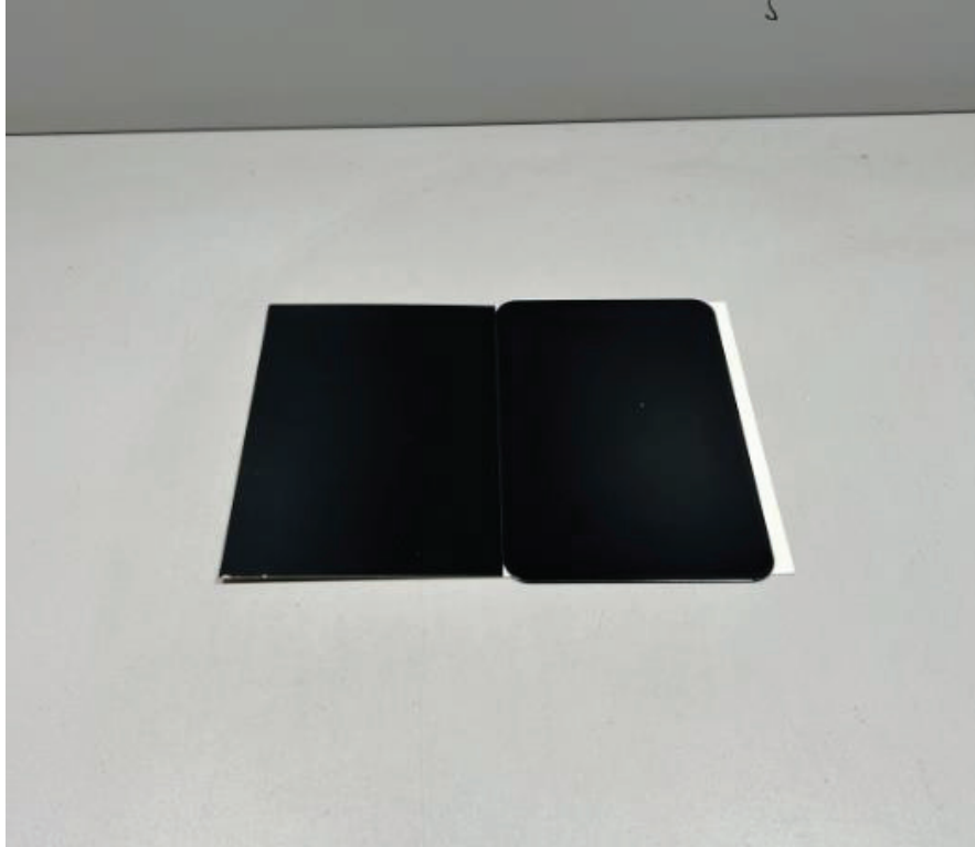
Figure 5.24. Color matching study of RAL 9011 (Left one is conventional RAL 9011, right one is color matching study with IR reflective pigments)
