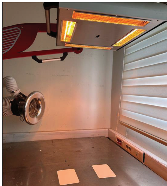
Figure 4. 5. IRT Model 4-1 PCD IR Heater
