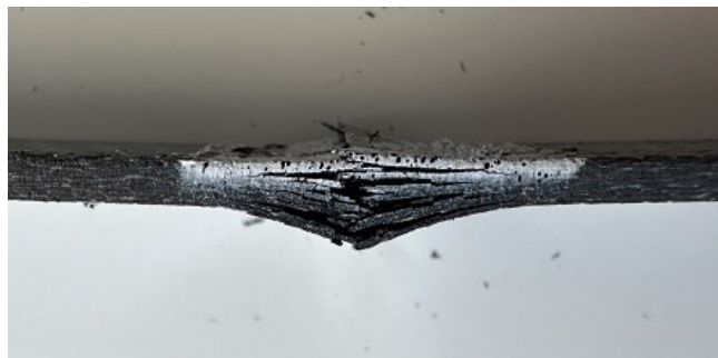
Figure 4.9. A picture of failed compression test sample in the weft direction
