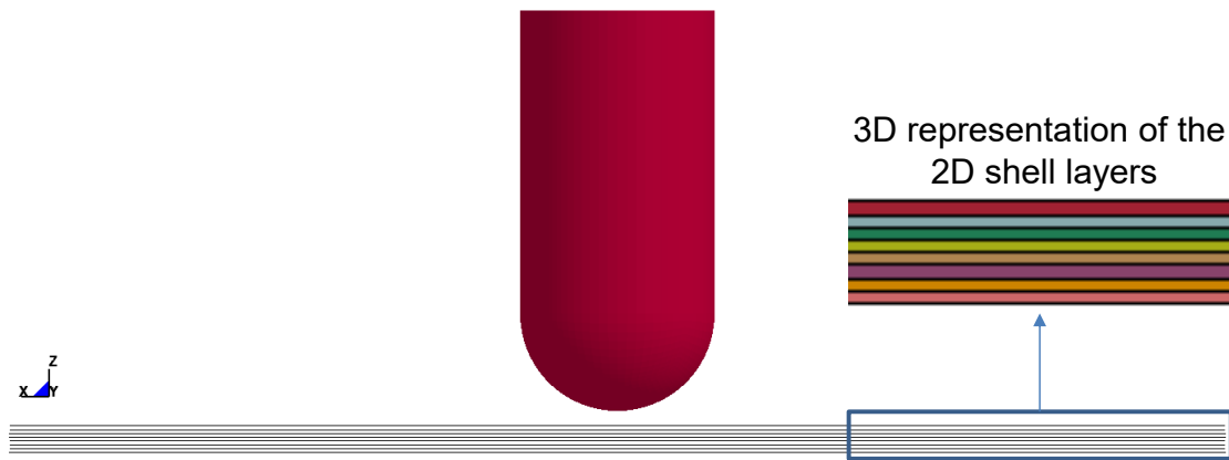
Figure 5.14. Finite element model of stacked shell drop weight impact testing
