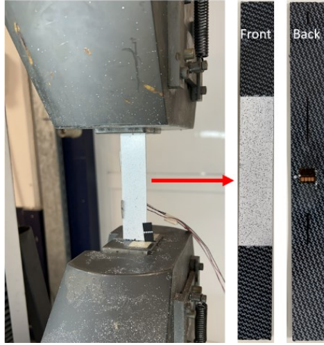
Figure 3.15. Standard in-plane shear test of \pm 45^\circ specimen test setup
