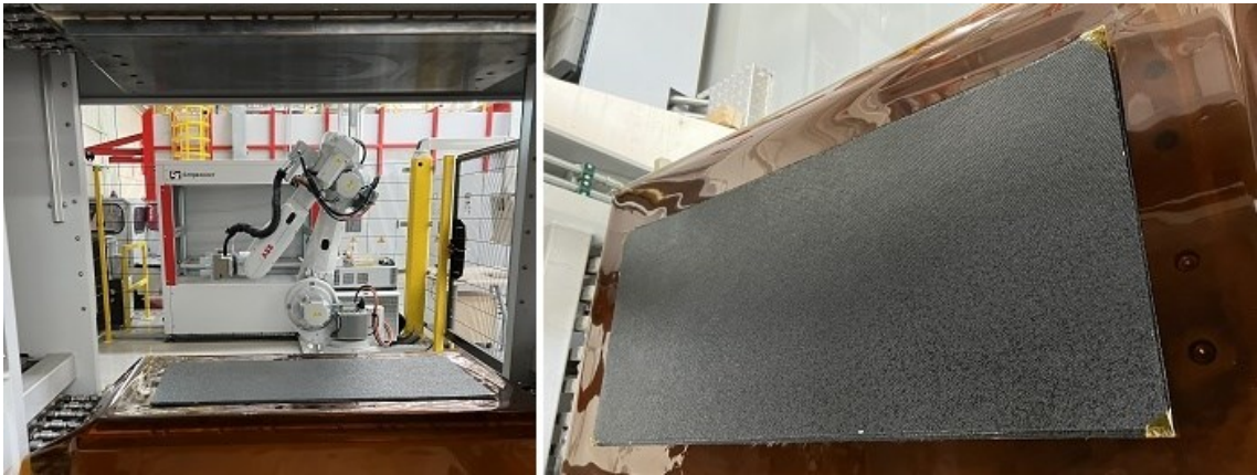
Figure 3.2. Composite laminate before consolidation process
