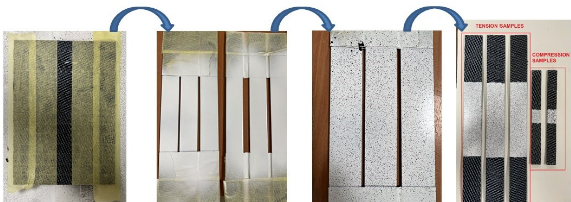
Figure 3.9. Specimen Surface Preparation for DIC Application
