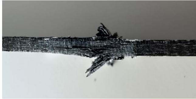
Figure 4.7. Failed compression test sample in the warp direction
