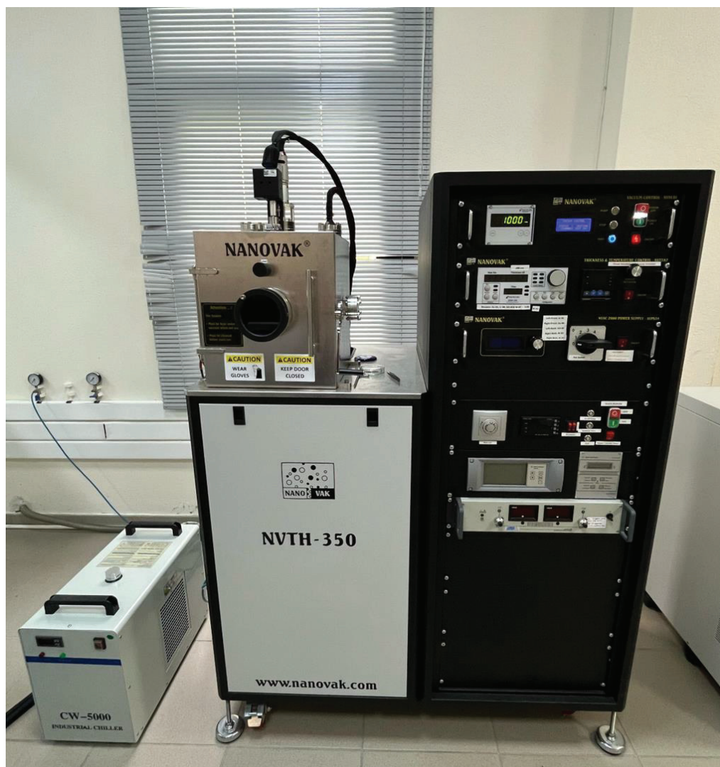
Figure 2.5. Nanovak NVTH-350 Thermal Evaporation System including Edwards. RV8 Turbomolecular Pump, Inficon VG401 Pressure Gauge, Ordell PC771 Temperature Gauge, SQM-160 Rate/Thickness Monitor, Pot Switch, 12V - 200A Sequential/Co-evaporation Thermal Evaporation Sources, Diener Electronic SS 304 Vacuum Chamber and CW-5000 Industrial Chiller in QDL.
