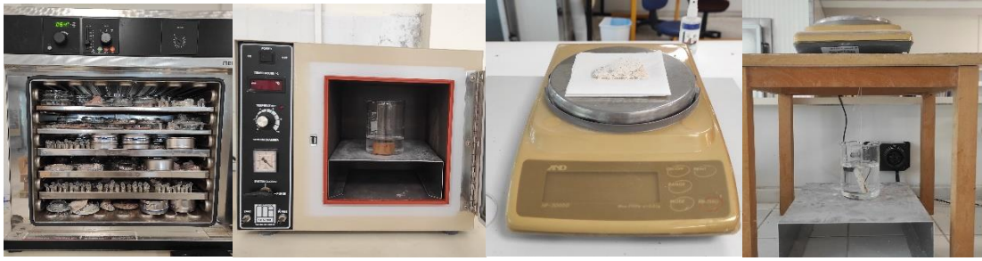
Figure 4. 6. a: Oven for drying samples b: Precision balance used to weigh dry and saturated samples c: Samples in vacuum oven d: Archimedes weight measurement
