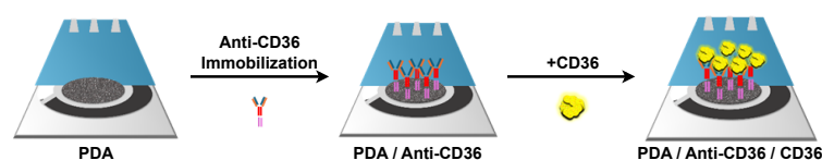
Figure 2.1. Schematic illustration of immuno-biosensor surface preparation.
