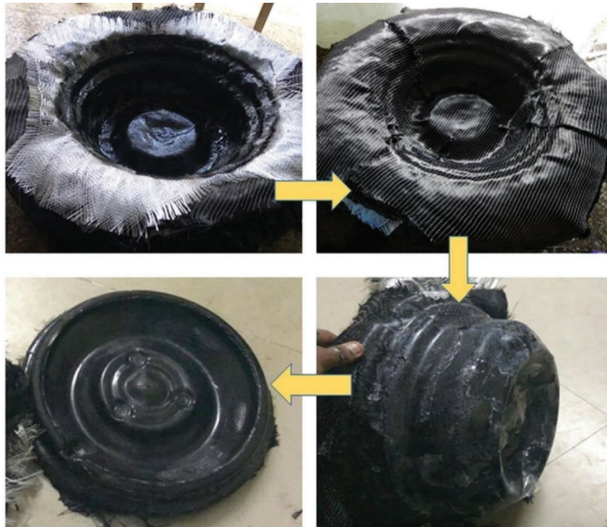
Figure 2.6. Preparation steps of polymer matrix composite wheel (Source: Edwin Raja Dhas et al., 2023)
