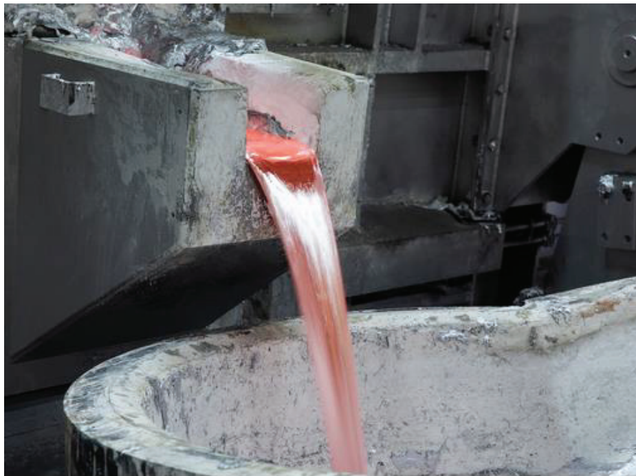
Figure 3.4. Molten metal transfer from melting furnace (“Cevher,” n.d.)
