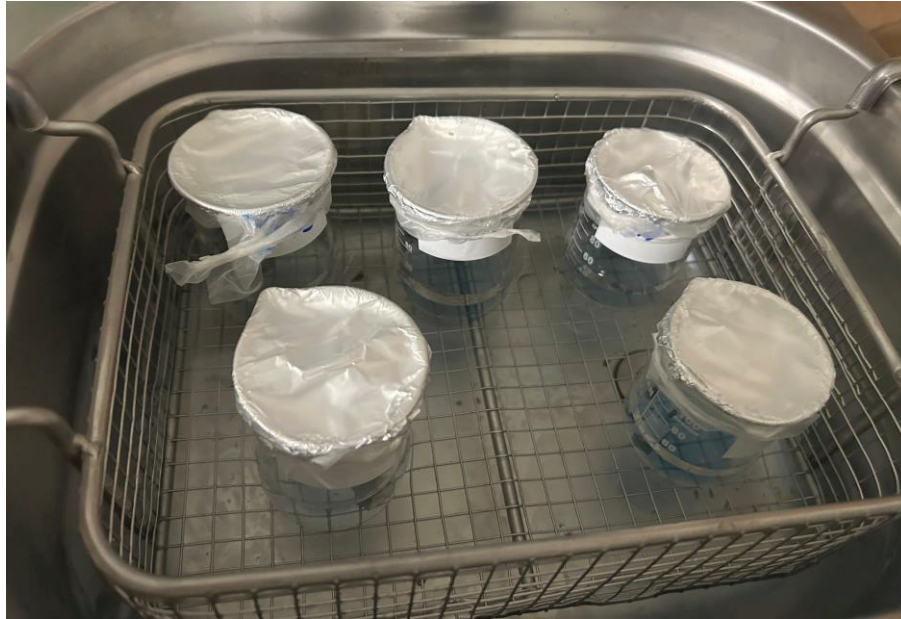
Figure 3.19. Ultrasonic cleaning of SEM samples
