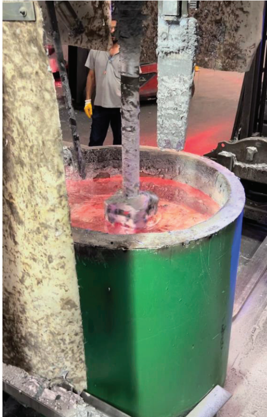
Figure 3.5. Rotary degassing operation
