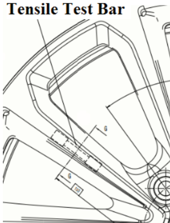
Figure 2.11. Technical drawing of the location for tensile test bar
