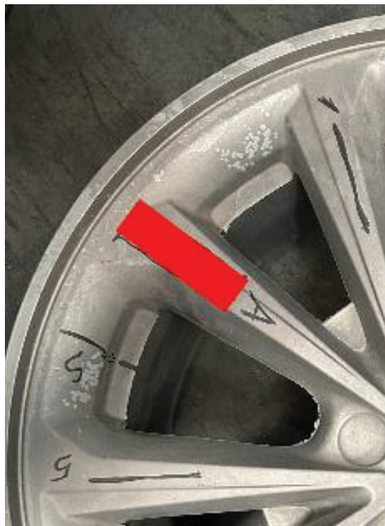
Figure 3.12. Red coloured Charpy specimen region on a wheel
