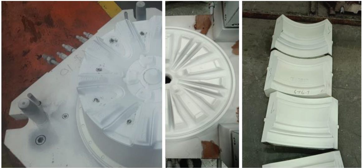
Figure 3.6. After mold coating operation
