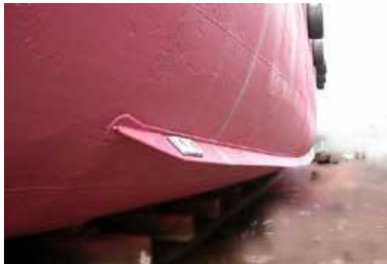
Figure 1.3. Bilge Keel on a Ship (Source: Sinha, 2022)
