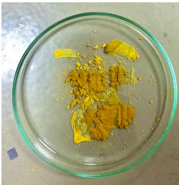
Figure 21. Decomposed fabric structure after in-situ dip coating process
