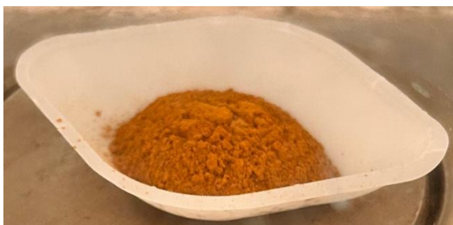
Figure 7. As synthesized Ni-MOF-74 powder (MOF-74(1:1))
