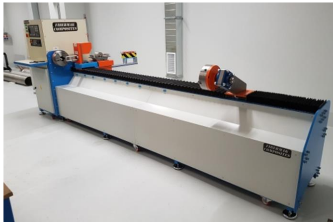
Figure 3.10 General view of 4-axis filament winding machine
