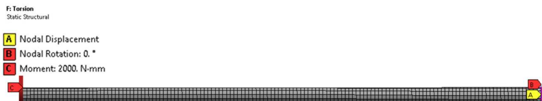
Figure 5.6 Boundary conditions of torsional stiffness model
