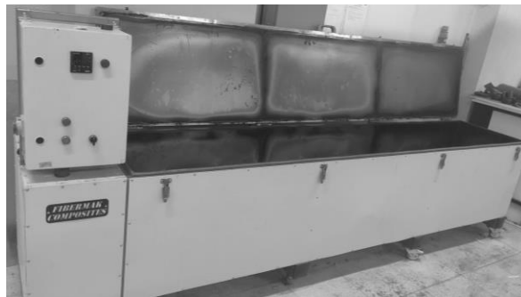
Figure 3.14 Rotating curing oven
