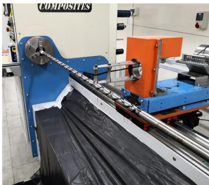
Figure 3.11 Production of [\pm 45]_6 lay-up composite rod
