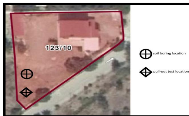
Figure 3.1 Location of the project site in Seferihisar (a) soil boring location (b) pull-out tests location
