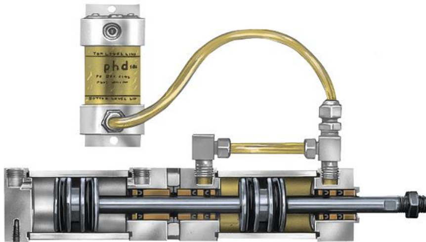
Figure 2.3. Example of Tandem Hydraulic Actuator (Source: Aerospace Actuators 2 19 )
