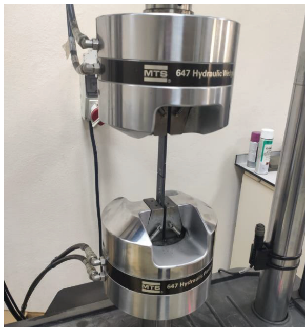
Figure 3.9. Fatigue test setup on the MTS Landmark™ Servohydraulic Test System
