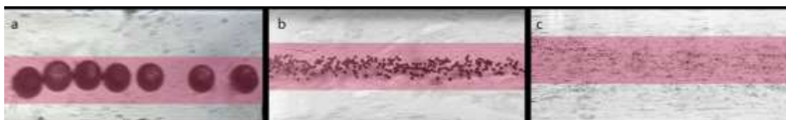
Figure 63. Comparison of PSMs with different sizes; A) 200 \mu\text{m} , B) 20 \mu\text{m} , and C) 5 \mu\text{m} with 100x dilution ratio.
