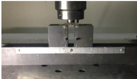
Figure 4.8. The test setup for three-point bending test
