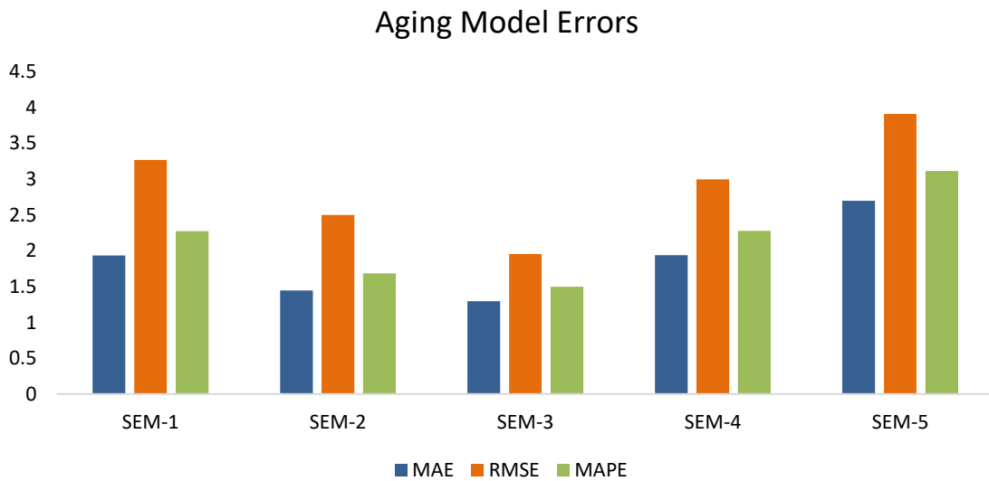
Figure 20. Performance indicators for each LFP dataset modeling with analytical solution.
