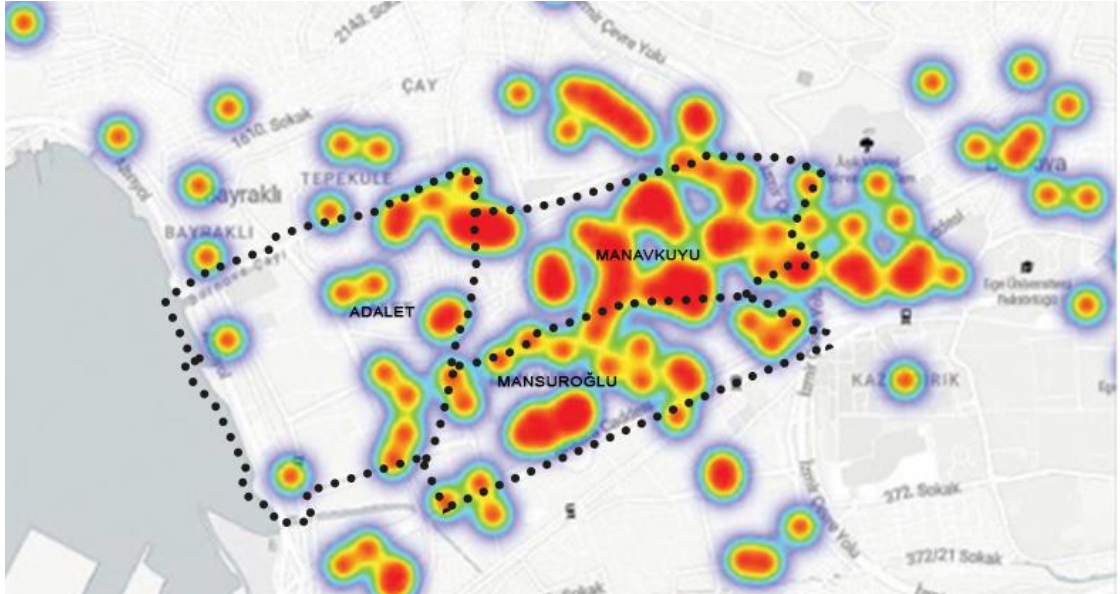
Figure 31. 30 October 2020 Earthquake Damage Intensity Map
