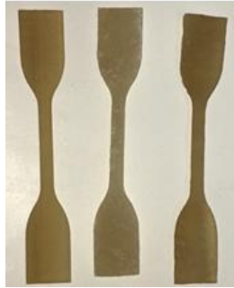
Figure 4.6. Extrudates with 30 wt.% glycerol content.
