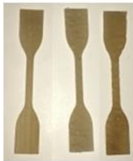
Figure 4.7. Extrudates with 40 wt.% glycerol content.
