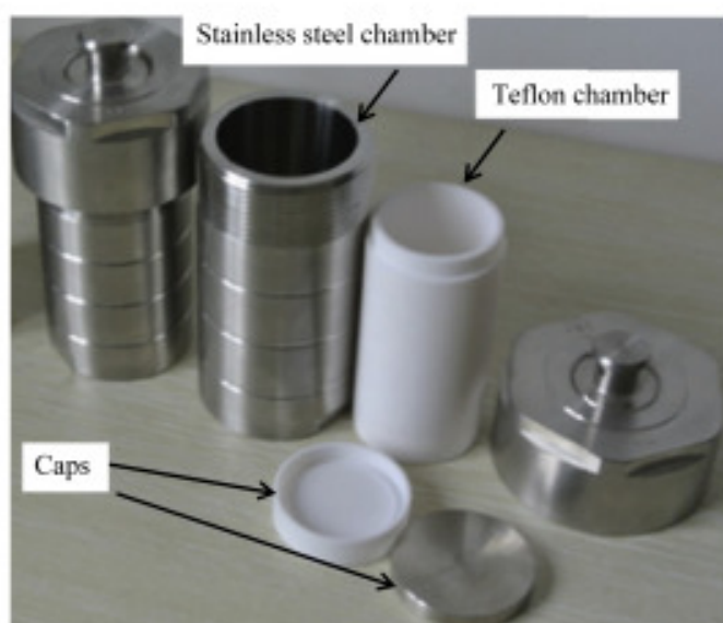
Figure 2.1. The main components of hydrothermal synthesis are the teflon-lined container placed in the autoclave and the solvent and precursor required for the experiment.
