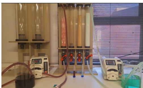
Figure 34. Resin experiment with IX column in a continuous process.
