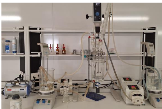
Figure 19. The batch crystallization experimental set-up.
