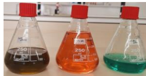
Figure 23. Feeding and output solution of process. Eluate, \text{CoSO}_4 , and \text{NiSO}_4 from left to right.
