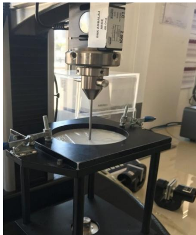
Figure 36. Puncture Resistance of 100% Mater-Bi® EF05B Measurement
