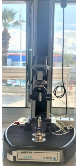
Figure 19. Equipment Tensile Strength and Elongation at Break test
