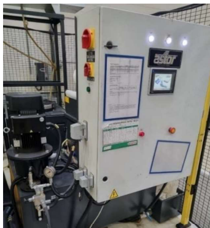
Figure 2.4. Image of Cooling unit of CNC Machine
