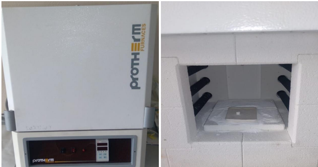
Figure 3.13. Demonstration of the muffle furnace used for decomposing the polymeric part of the solution.
