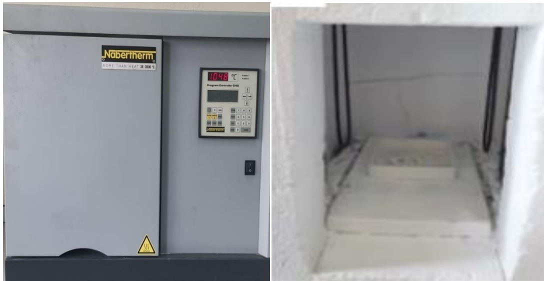
Figure-3.10. Laboratory kiln for sintering and bisque firing pellets
