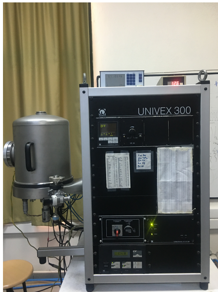
Figure 3.16. IZTECH physics department's lab thermal evaporation system.
