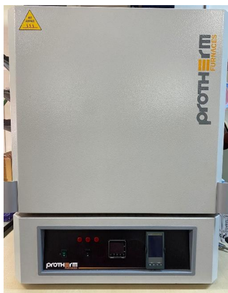
Figure 3.3. Protherm laboratory-scale electrical resistance chamber furnace.
