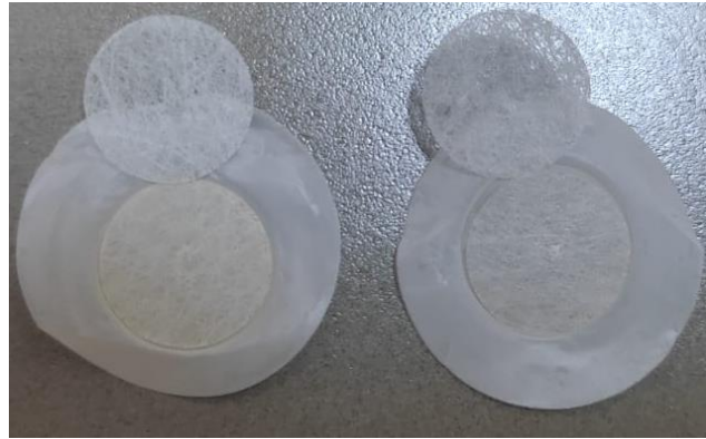
Figure 35. Polycarbonate membrane color changes after the extrusion process (left polycarbonate membrane: 0.018 TRQ/Lipid molar ratio, right polycarbonate membrane: 0.006 TRQ/Lipid molar ratio).
