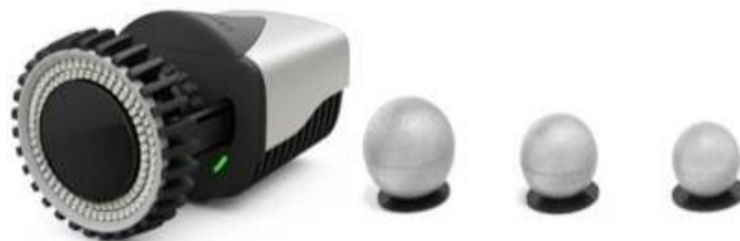
Figure 15. Miquis M3 Camera and Reflective Markers
