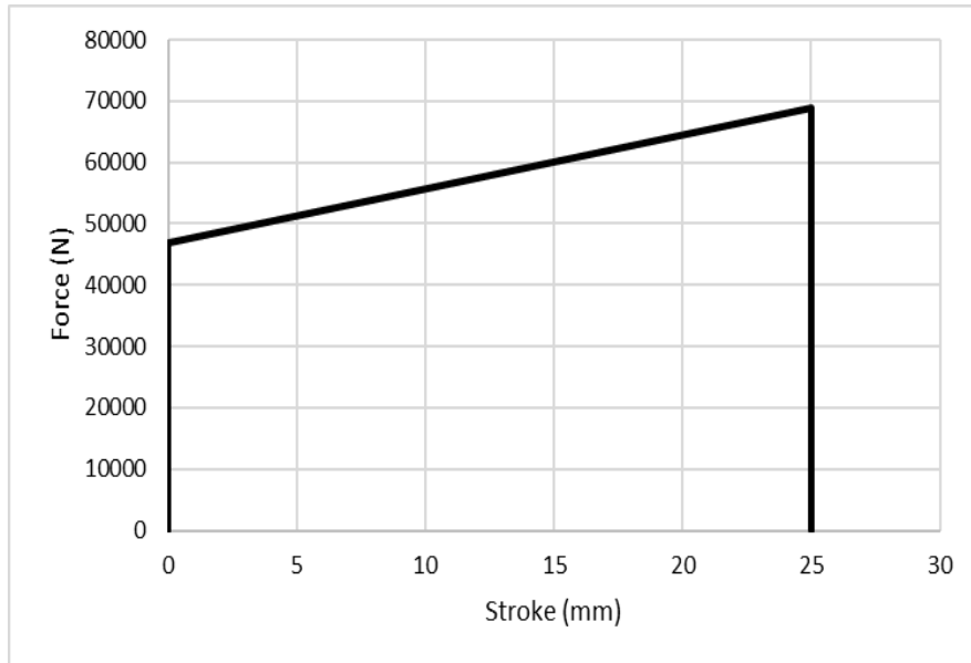
Figure 40. Characteristic Load Curve for Gas Springs
