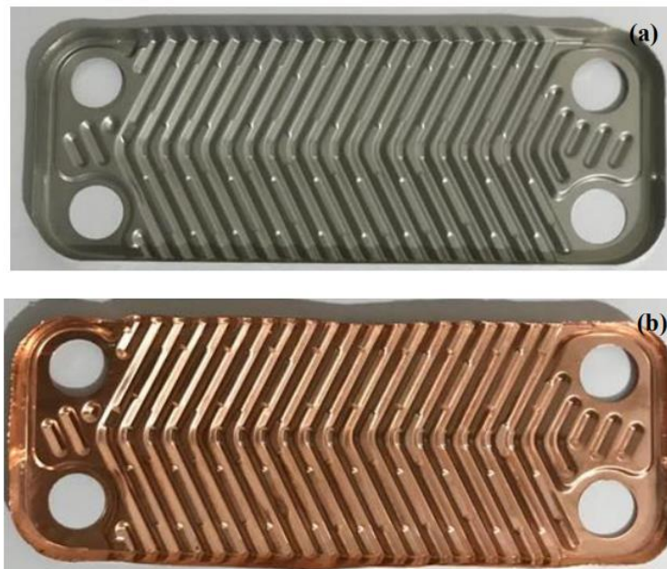
Figure 14. PHE Plate (a) and filler material (b) (Source: Hayta, Y., 2020)
