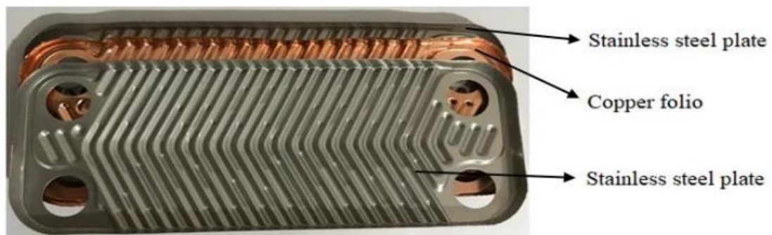
Figure 6. Copper foil (filler material) between two stainless steel channel plates (Source: Hayta, Y., 2020)
