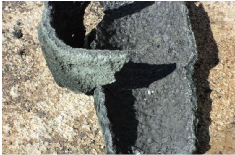
Figure 2. 3. Fe, Mg silicate deposit obtained from Tuzla Geothermal Power Plant.
