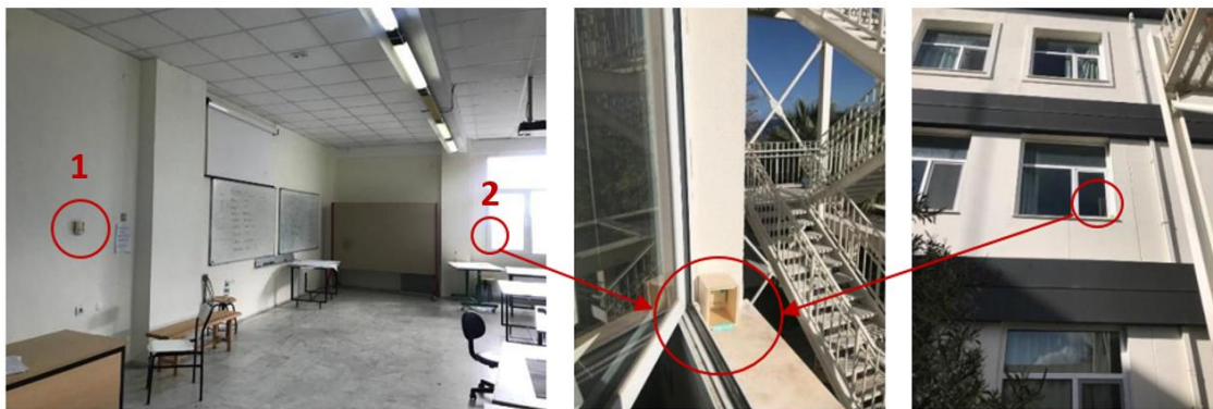
Figure 3.6. Photos of inner and outer climate data loggers (1: indoor, 2: outdoor)
