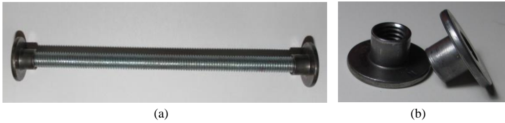
Fig. 1. Shear studs: (a) A single shear stud; (b) T-section nuts
