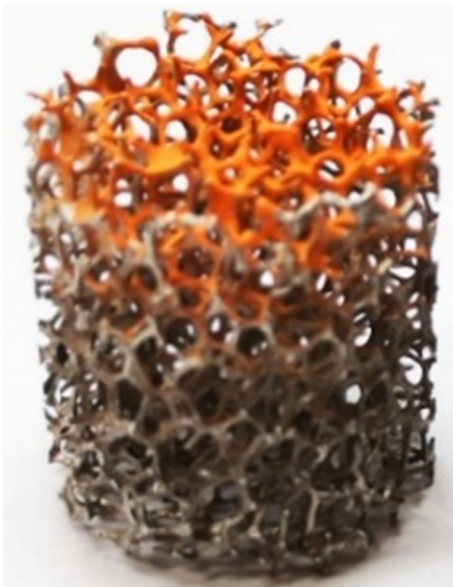
Fig. 1 – M-pore® open-cell aluminium specimen.
